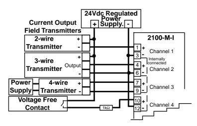
Connection configuration for 2 wire, 3 wire and 4 wire transmitters, and digital inputs.
