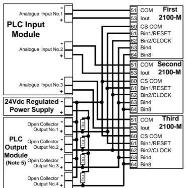
Connection of a 2100-M to a PLC with open collectors commoned to 0V of an external power supply.
