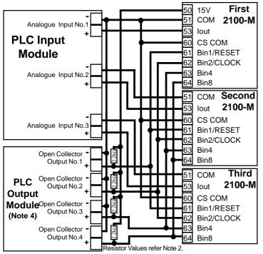
Connection of a 2100-M to a PLC with open collectors commoned to COM of the first 2100-M.
