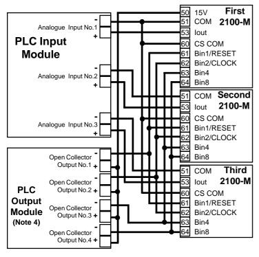
Connection of a 2100-M to a PLC with open collectors, commoned to the 15V of the first 2100-M power supply.
