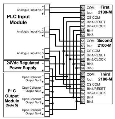
Connection of a 2100-M to a PLC with open collectors, commoned to +24V of an external power supply.
