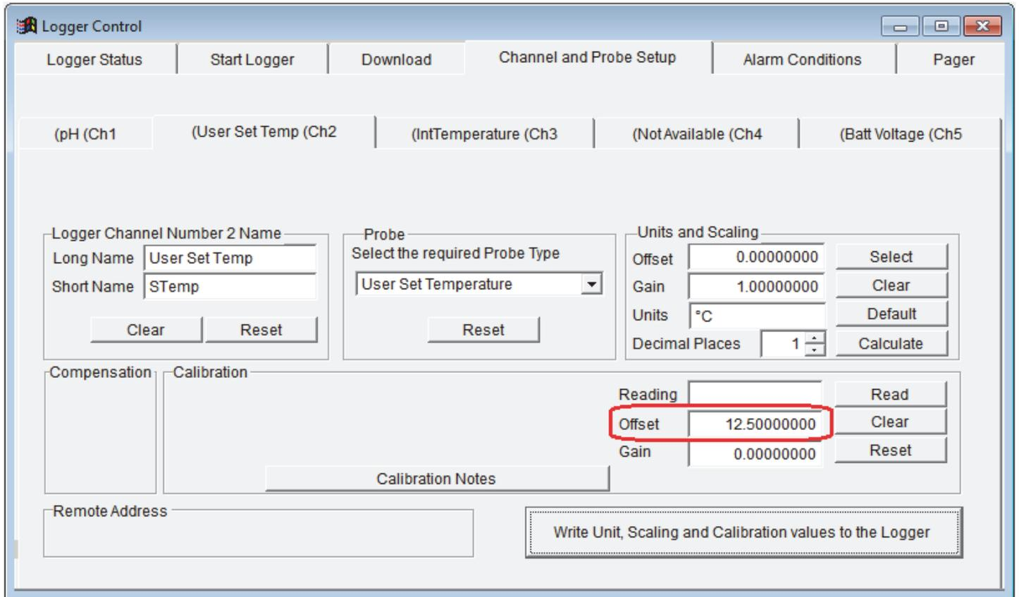
The logger will now operate with the temperature set to the value entered in the Calibration Offset box and temperature compensation will be applied at this set temperature. Realtime read and Logged data will show the set temperature as shown below:
