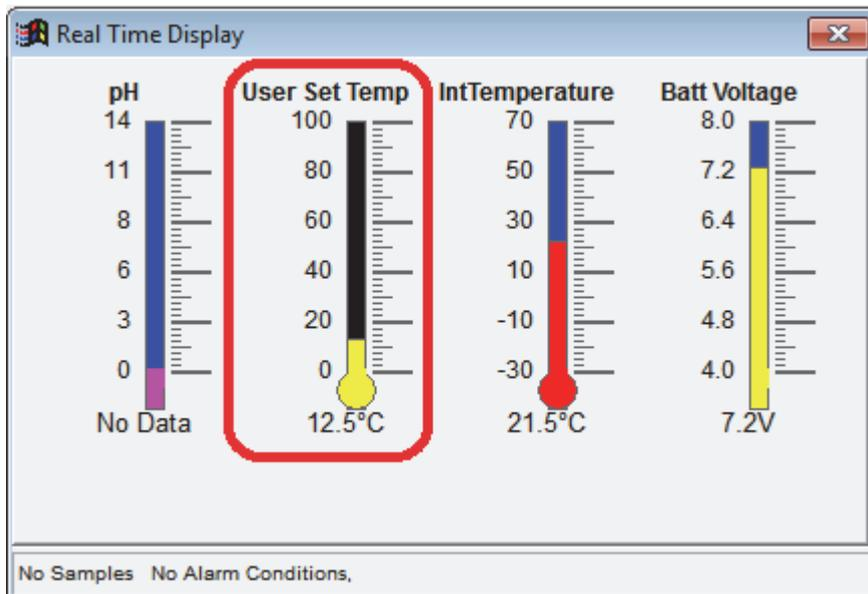
The User Set Temperature can then be changed at any time by entering the new value in the Calibration Offset box and then click the "Write Unit, Scaling and Calibration values to the Logger" button.
